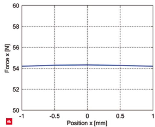
6 Measured forces of in-plane motor. (a) Force versus current. (b) Force versus position at  $I = 2.5$  A.
