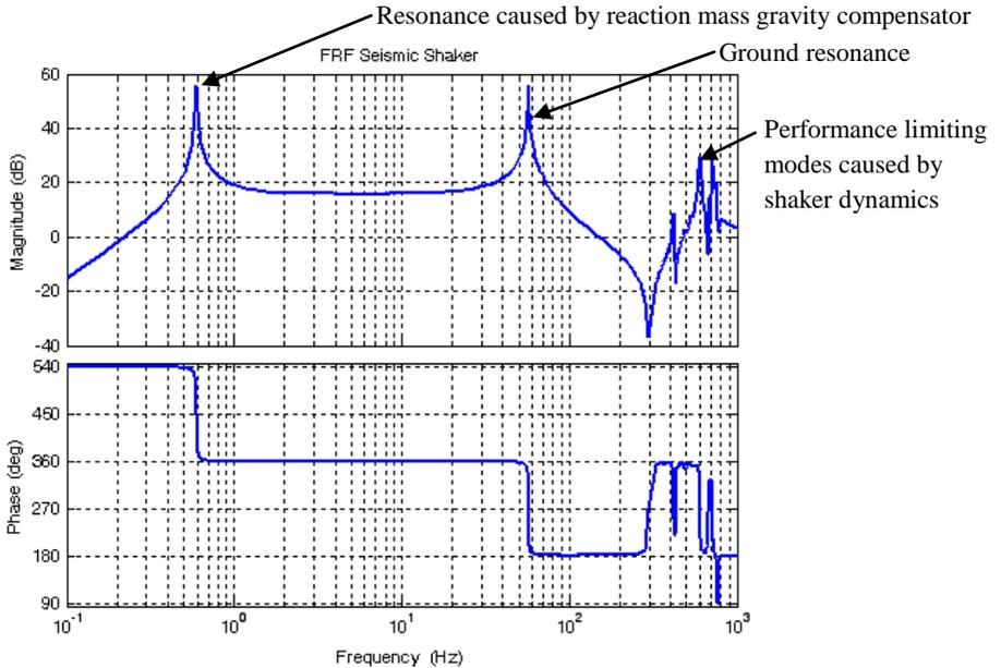
Figure 3: Typical FRF of seismic shaker: input actuator force, output ground force
