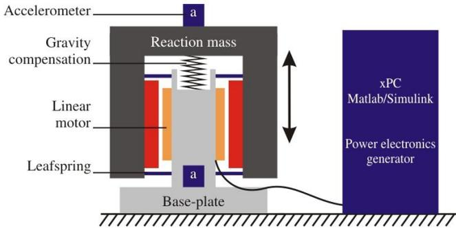
Figure 2: Proposed seismic shaker for seismic monitoring using linear motors. The gravity compensator of the reaction mass consists of a static air bellow. The guiding is realized with parallel leaf springs.
