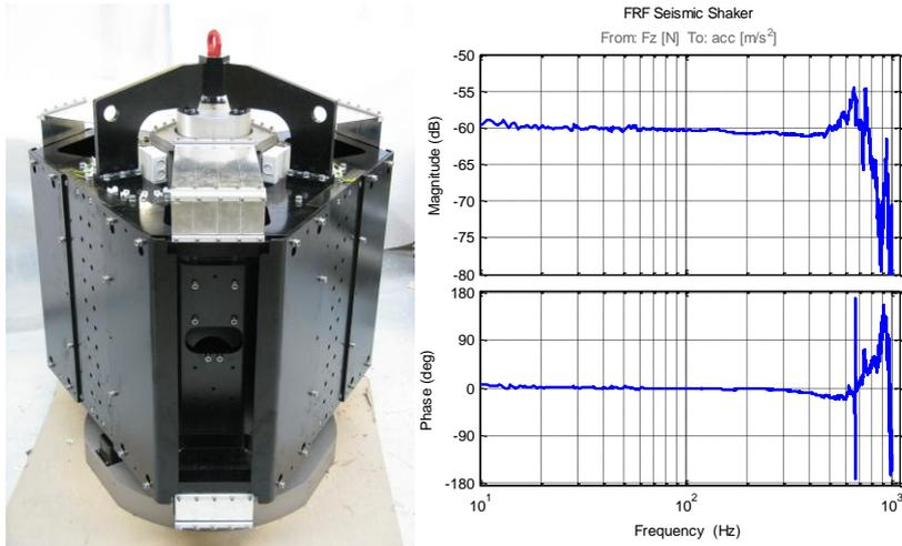
Figure 4: Assembled seismic shaker and FRF of the reaction mass
