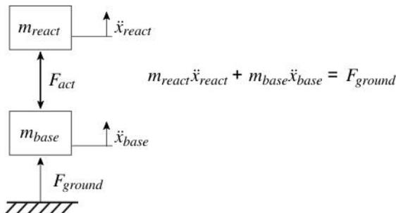
Figure 1: Dynamic model of a seismic shaker
