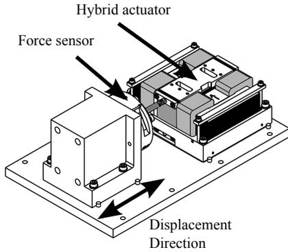
Figure 10: Setup to measure static forces of the hybrid actuator.
