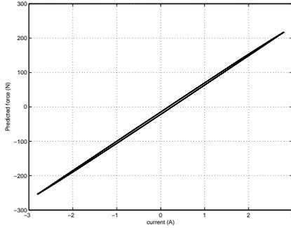
Figure 15: Force predicted using integrated hall sensors
