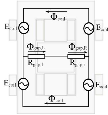
Figure 5: Magnetic equivalent network of the hybrid actuator for the coil circuit. Stator and mover material are assumed to have negligible reluctance.
