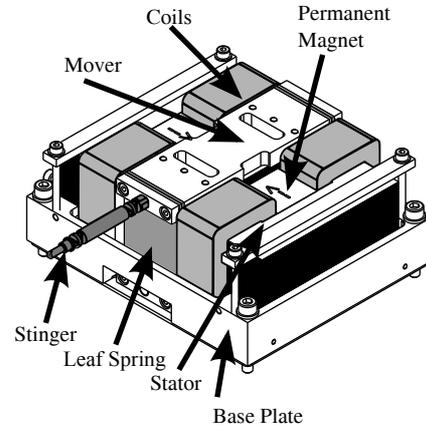
Figure 9: Hybrid actuator in its mechanical assembly. A linear encoder to measure the position of the mover is present at the bottom of the mover (not visible in image).
