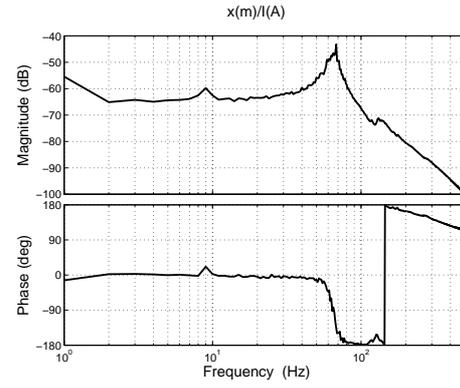
Figure 16: Plant FRF of hybrid actuator
