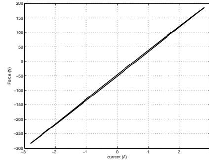
Figure 13: Current vs force at center of air-gap for oriented core material, a hysteresis band of 4 N is present
