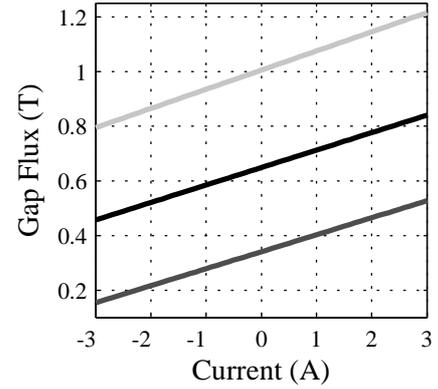
Figure 8: Flux density of the right air gap when generating the force from Fig. 7. The figure shows the flux density with the actuator in -1 mm position (—), Actuator in 0 mm position (—), Actuator in 1 mm position (—)
