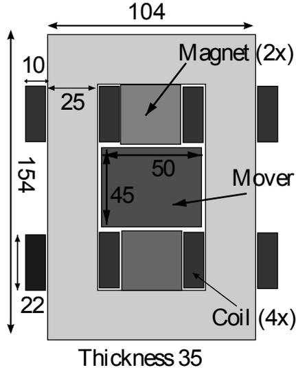
Figure 3: Dimensions of hybrid actuator to be used as reaction force cancellation actuator. The actuator is capable of generating 300N with 300 At in total. The lamination of the stator and mover is stacked perpendicular to the image.
