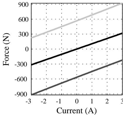
Figure 7: Force generated by the actuator. The figure shows the force with the actuator in -1 mm position (—), Actuator in 0 mm position (—), Actuator in 1 mm position (—)
