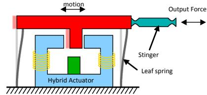
Figure 2: Hybrid actuator with a parallel plate spring guide to compensate for actuator stiffness and to constrain the other 5 Degrees of Freedom. The stinger transfers the force to the isolated platform
