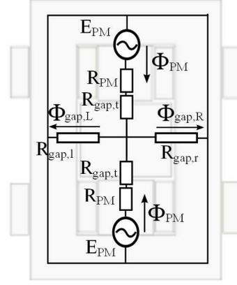
Figure 4: Magnetic equivalent network of the hybrid actuator for the permanent magnet circuit. Only the magnetic reluctances of the air gaps and permanent magnets are included, stator and mover material are assumed to have negligible reluctance.
