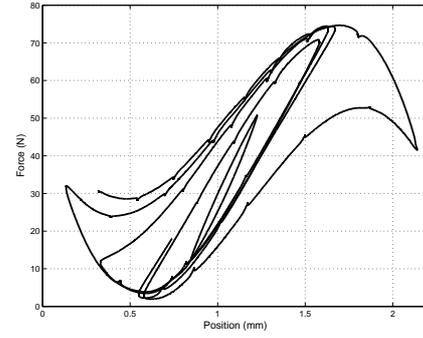
Figure 11: Position vs force close to the centre of air-gap for oriented core material, the zero position is where the actuator is stuck at end stop attached to the stator. In the center the stiffness is dominated by the plate springs and is positive.
