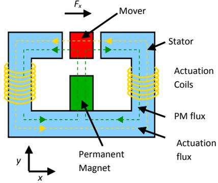
Figure 1: Hybrid actuator creates a force in x direction on the mover. The permanent magnet generates a bias flux which can be manipulated with the coils.
