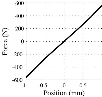
Figure 6: Negative stiffness of the magnetic design of the actuator. This stiffness will be compensated by the parallel plate spring guide.
